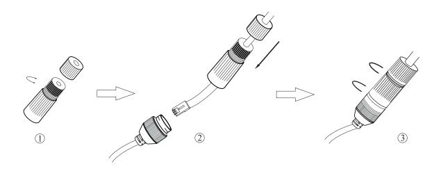
**Step 1:** Loosen the nut from the main element.
