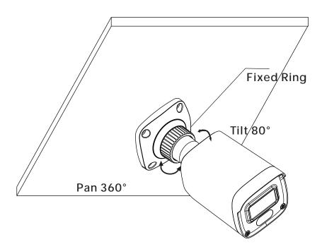
**Step 6:** Tighten the fixed ring after the adjustment.
